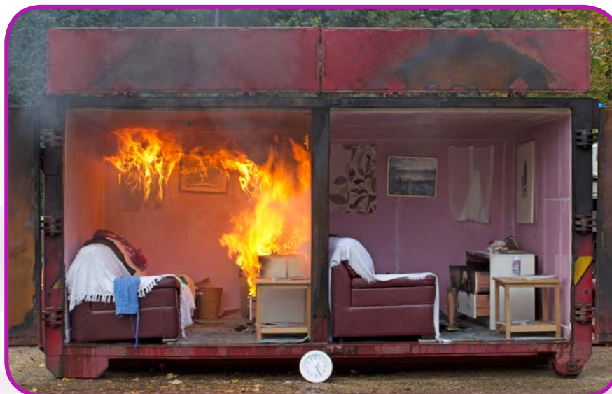
Sprinkler activation demonstration, showing a room set with no sprinkler on the left and a room set fitted with a sprinkler on the right
